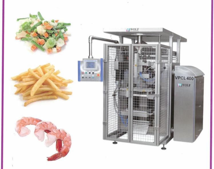
Entirely made of stainless steel, wash down and IP 65, are just some of the keyfacts of our baggers dedicated to the frozen food or liquid industry. Up to a bag width of 450mm, The Wolf stainless steel baggers, can handle heatsealable laminates, as well as plain LDPE on speeds of up to 120B/min.
