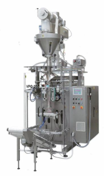
Powder is probably the most difficult product to fill into a flexible bag on a descent output rate! To achieve the highest filling accuracy and highest output speed, the auger feeder, and vertical bagger from Wolf, which are all made according to the highest hygienic standards, cover both. Participate of our experience in powder filling for more than 25 years.
