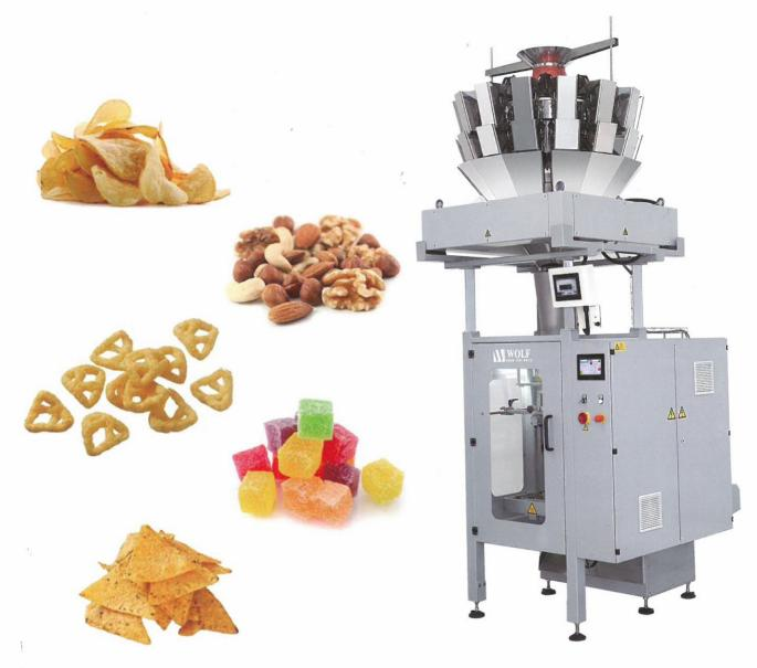
The EPS model has been especially developed for packing snacks, candy, nuts and similar products. The body frame is designed to integrate a multiheadweigher and a inline metal detector on the smallest floorspace possible. This fully servo driven continuous motion bagger does pack extruded snacks on speeds up to 130B/min, and potato chips up to 100B/min.
